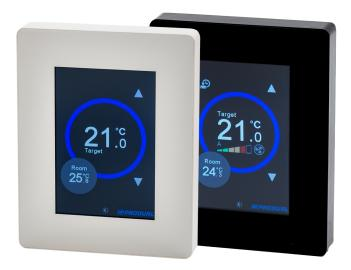
TRI-P-1R touchscreen room units provide attractive user interface and sensor for room control applications. The devices are connected to BMS or controllers via Modbus or BACnet communication interfaces. The room units have  $320 \times 480$  pixel 255 colour touchscreen that displays the plant and control status information on the modern intuitive user interface.
