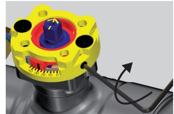
Lock again and re-open the valve. Overtightening could seriously damage the device. Max. torque used: 2-3 Nm.
