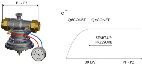
Using a differential pressure gauge to measure the pressure drop the valve absorbs allows checking whether the valve is in the operating range (and, therefore, whether the flow is constant) by simply verifying that the measured value P1 - P2 is higher than the start-up value.
