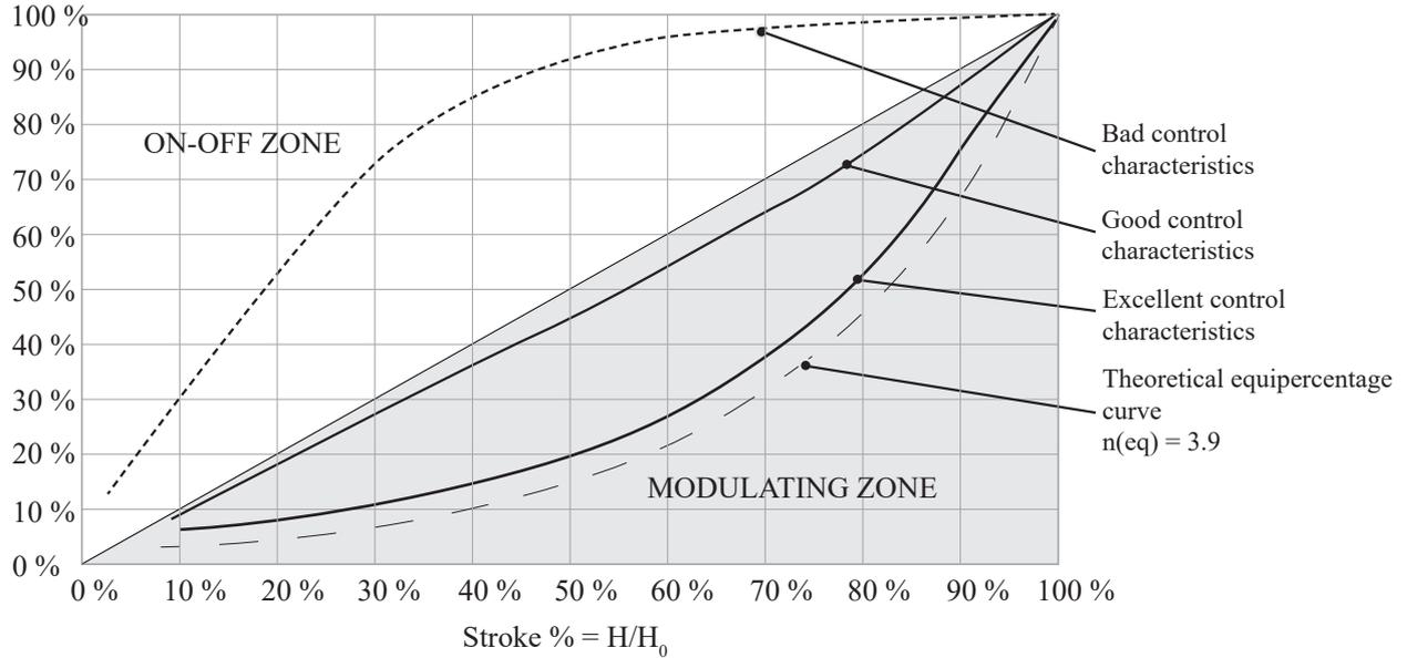
Combining the PCMTV valve characteristics with heat exchanger results in a linear control system.
