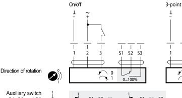
Connected with conductors S1, S2 and S3 (only model RDAB5-230S)
