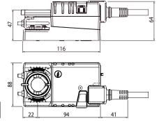
Damper spindle Length O±♦ min. 37 6 ... 20
