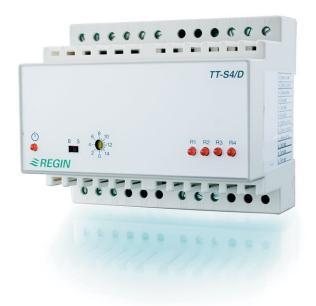
TT-S4/D is a micro-processor based step controller for controlling cooling or heating applications. The step-controller is controlled by a 0...10V signal from a TTC25/TTC40F or another controller/ DDC.
